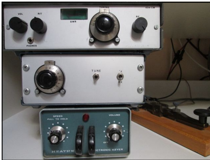
Top: 40 meter transceiver. Middle: VXO CW transmitter for 20 meter. Bottom: Heath keyer; on the right a handmade straight key (by PA2JS, as a gift for teaching him the morse code)
