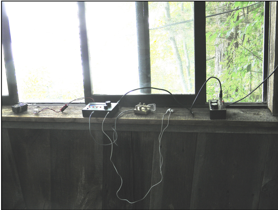
From left to right are the battery pack, R4020, key, ear buds, tuner, antenna feed.
