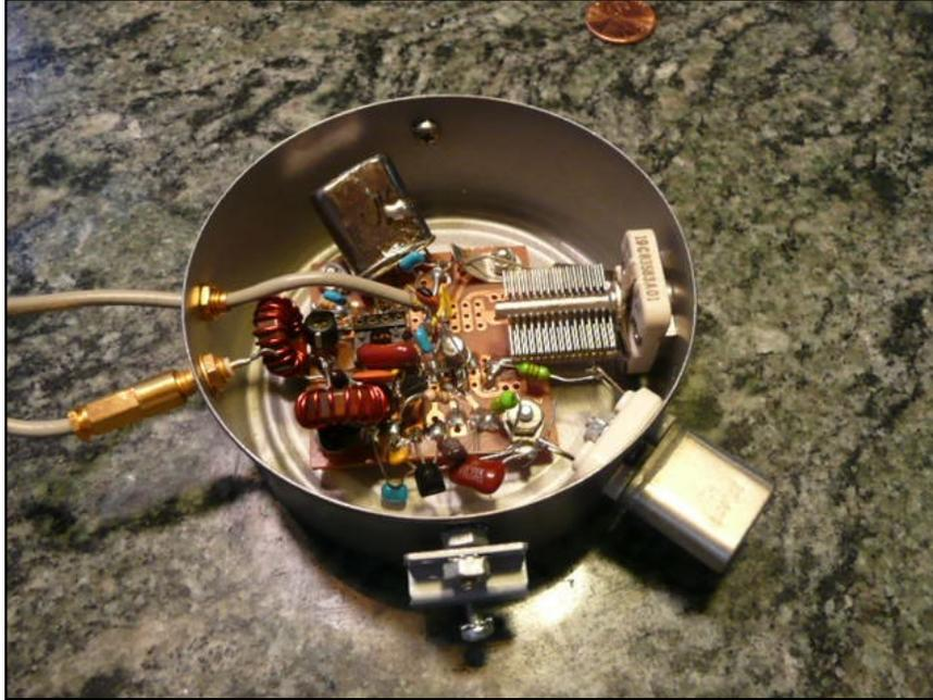
The third pic shows a tube transmitter built into a prune tin, fittingly named "Pruna-Tin". The tin is somewhat taller than the large tuna tin, even though it is labeled "9 oz.". It's a crystal controlled 15MF8 triode/pentode compactron tube powered by an old Heath HP-23A power supply.
