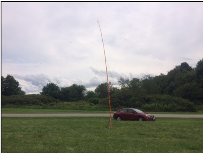
Mike's (L) and John's (R) inverted V jumper dipole antennas:
