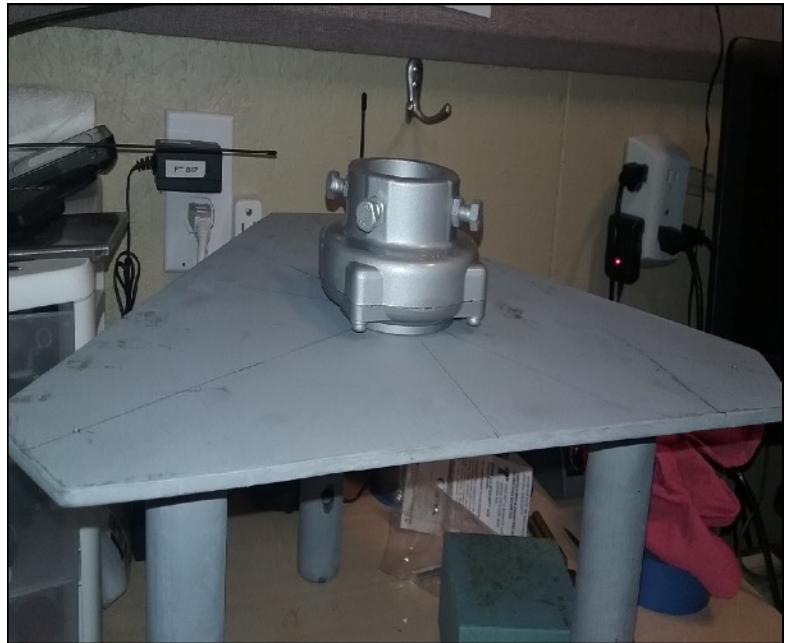
Home Brew Tower Cap for Thrust Bearing 1/4" plate Steel with a 2" thrust Bearing
