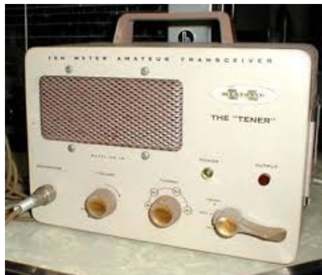
TENER : Heathkit, a ten meter transceiver with superregenerative receiver, brother to the TWOER and SIXER, aka the " Benton Harbor lunch boxes ".
