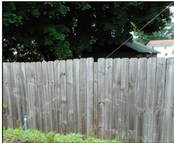
The far end of one leg of the dipole fastened to the blue pole.
