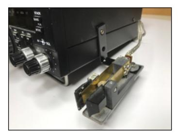
Looking at pics of other QRP rigs shows most also have cabinet or foot screws in suitable locations for a bracket. Try it on your next portable outing!
