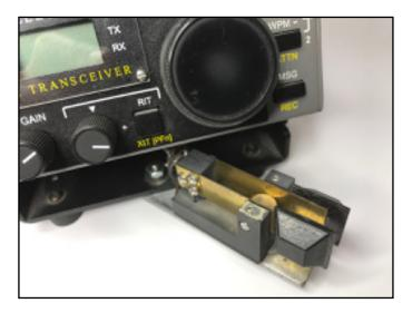
Later I constructed a set of micro-iambic paddles for the K1. These mount on the right front of the rig (second pic) using an existing cabinet screw hole. A small strip of double-sided plated circuit board was used as the center contact, and parts from an old relay were used for the arm/spring/contact assembly.
