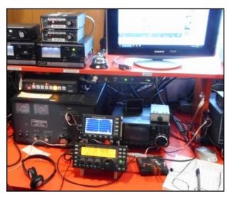
That's L-R: WB3FAE K3WWP KC2EGL and Bob WC3O from Skyview. Then my setup in their radio room where my KX3/PX3 combo is dwarfed by their big rigs. On top of their amp is a great antenna switching setup whereby any of their antennas can be connected to any of their operating positions. There is a computer driven lockout that prevents a position from connecting to an antenna that is in use at another position.
