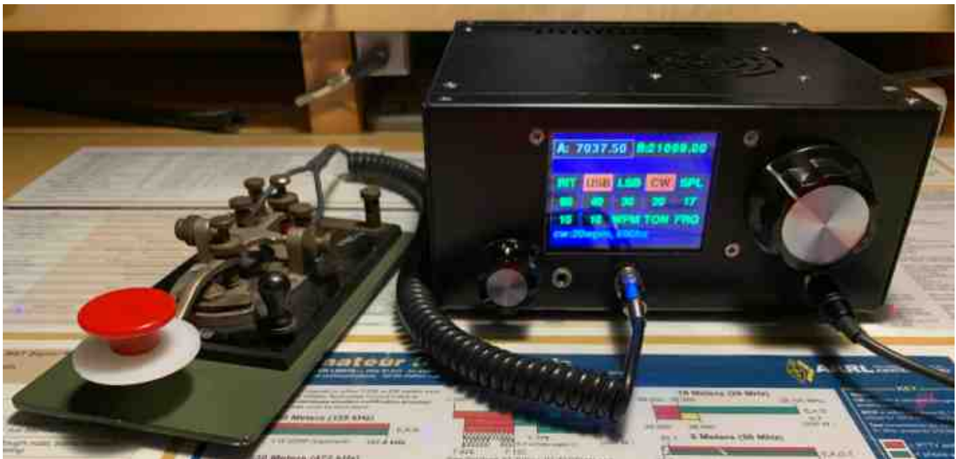
The latest project: A uBITX V6 and a J-38 key
