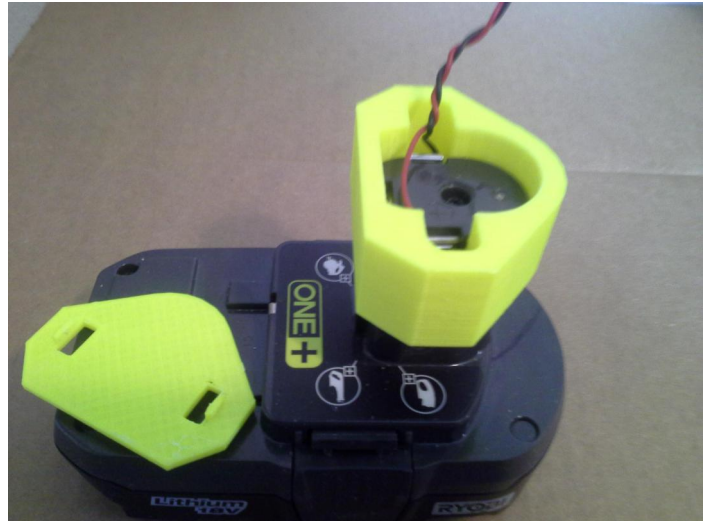
2-piece 3D printed Ryobi battery adapter
