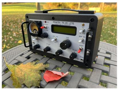
radio's case provides a nice sound chamber. The TR-45L comes with a couple of options, neither of which I chose to add to my order. One is a built-in rechargeable battery (5200 mAh), and the other an antenna tuner. I have plenty of batteries, and normally use resonant antennas.
