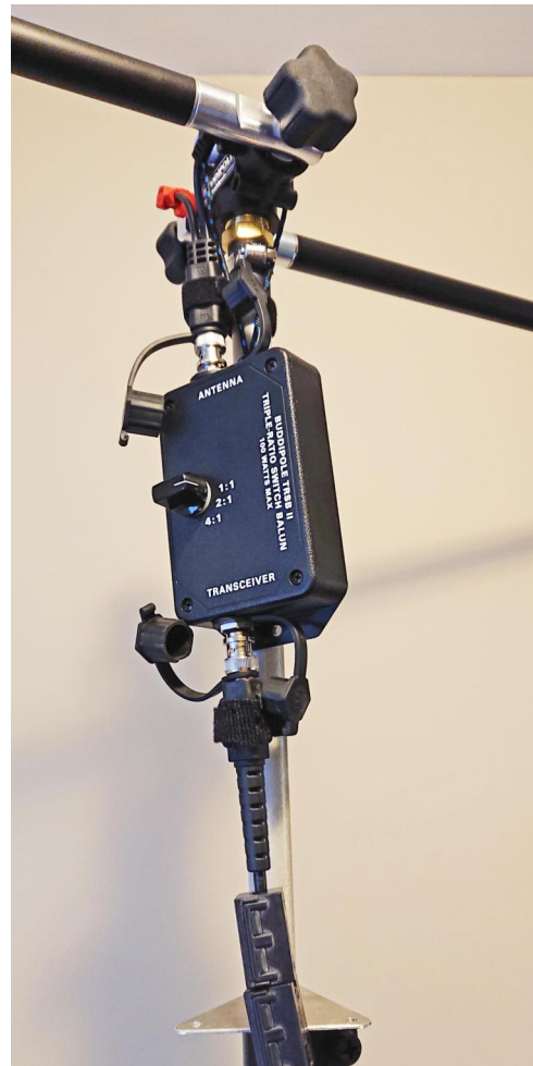
Finished installation with heat-shrink and hose clamp added, also showing my aluminum guy attachment plate
