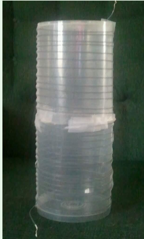
My crude "extra loading coil" (wound on CD boxes) that allows using the wire on 160 meters.
